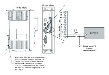
Figure 12: Epsilon Auxiliary Power Supply Wiring Diagram
